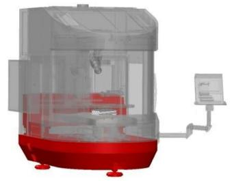
Figure 1: Polymer Granite Base & Welded Steel Frame
